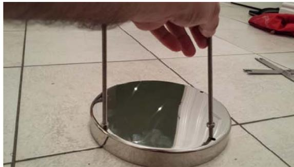
Rest threaded rod on the base plate (with flat top facing upwards) while tightening the other end of the rod with another nut from underneath of the base plate
