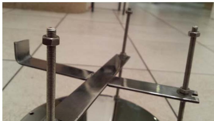
Adjust remaining 3 nuts on each rod as shown above. Make sure these nuts are equally spaced on the threaded rods as these will be used to rest top plate
