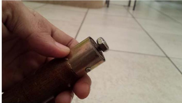
Unscrew the nut from wooden handle & attach it with the top plate (with 3 big holes) from the centre hole
