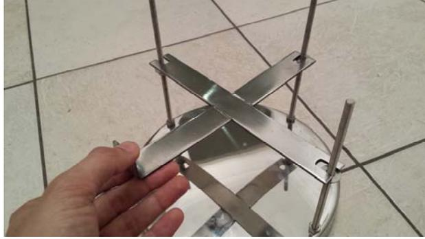
Rest the bracket on the washer and drop 1 x washer then tighten 1 x nut to secure the bracket
