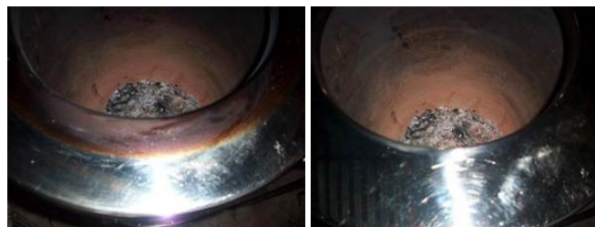
Mouth of Tandoor with cooking residues , cleaned with stainless steel cleaning solution
