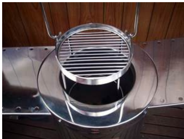
Stainless steel bbq grill being lowered into Tandoor using "U" ends of the naan rods
